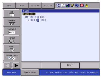
The shock detection alarm in teach mode and play mode can be reset by the following operation.
