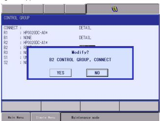
Select {YES} to set the system parameters automatically according to the selected items in the windows so far. Modification of System ConfigurationAddition of Base and Station Axes
