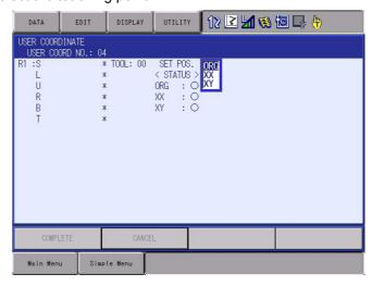
3. Move the manipulator to the desired position with the axis keys.
