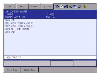
2. The next time an attempt is made to register the same instruction as in 1, the same additional items as were registered last time are also shown in the input buffer line.
