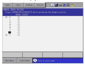
BRAKE STATUS O: Brake locked ●:Brake released
