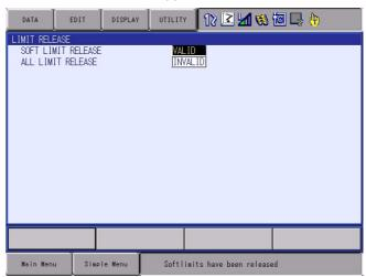
When "SOFT LIMIT RELEASE" is set to "INVALID", the message "Softlimits off released" is displayed for a few seconds.
